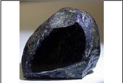
Figure 13. A black metamict zircon that is radioactive from its U-content Photo credit: GRR
