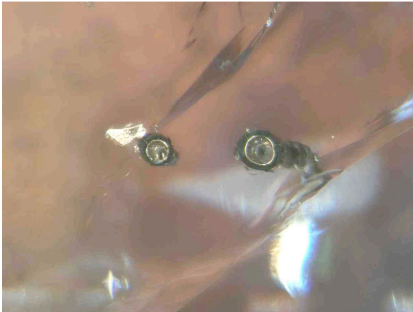
Figure 1. Two of the three pits exposed on the polished surface of the benitoite electron microprobe standard. The total width of the pit and the dark area surrounding it is close to 0.1 mm. Stacked images using Helicon Focus software provides the depth of focus.
