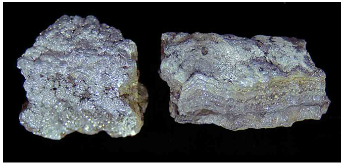
Galena-sphalerite scales from geothermal wellhead. Field of view is 9 cm wide.
