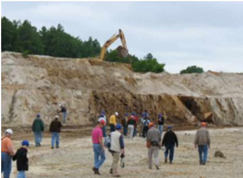
In the pit at the Archdale mine, Kings Mountain district, NC. White material is the weathered granite "ore." Dark material is older schist included in the granite intrusion. Paul Gordon photo.
