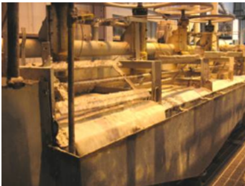
In the Zemex Industrial Minerals processing plant, mica flakes are separated from ground quartz and feldspar in floatation tanks. Paul Gordon photo.
