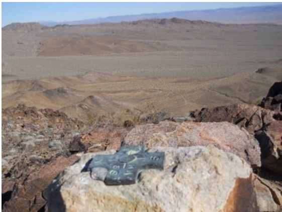
Brass USGS Mineral Survey marker 58 set in solid rock at high point with molten lead. (Wes Gannaway photo)
